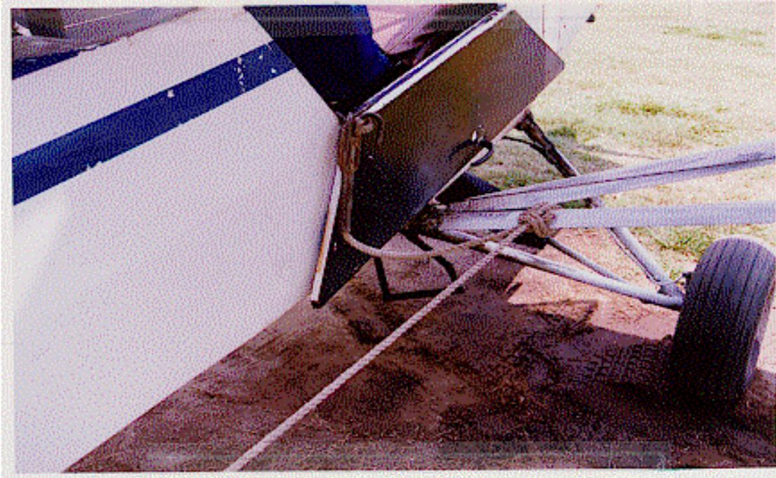
**FIGURE 2-4. EXAMPLES OF MULTIPLE GRAPPLE HOOK INSTALLATION**
