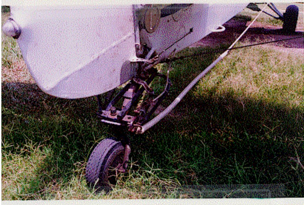
**FIGURE 2-2. EXAMPLES OF A VEE BAR**
