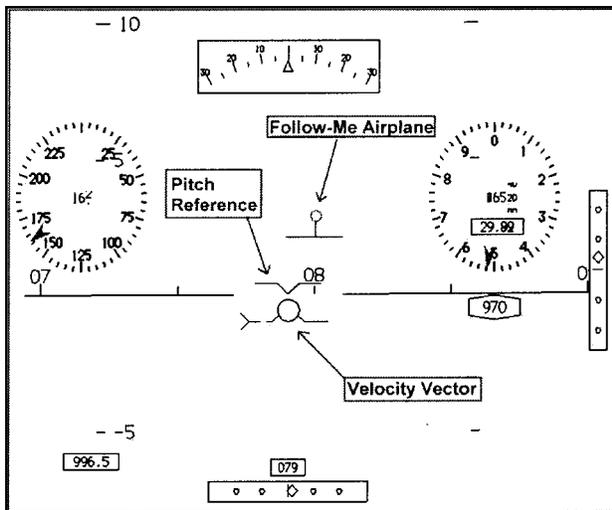
**Figure 2.** Display guidance symbology used in the experiment. Note that under the 'no-guidance' condition, only the pitch reference symbol was visible (from Beringer, 1999, reprinted with permission of author).
