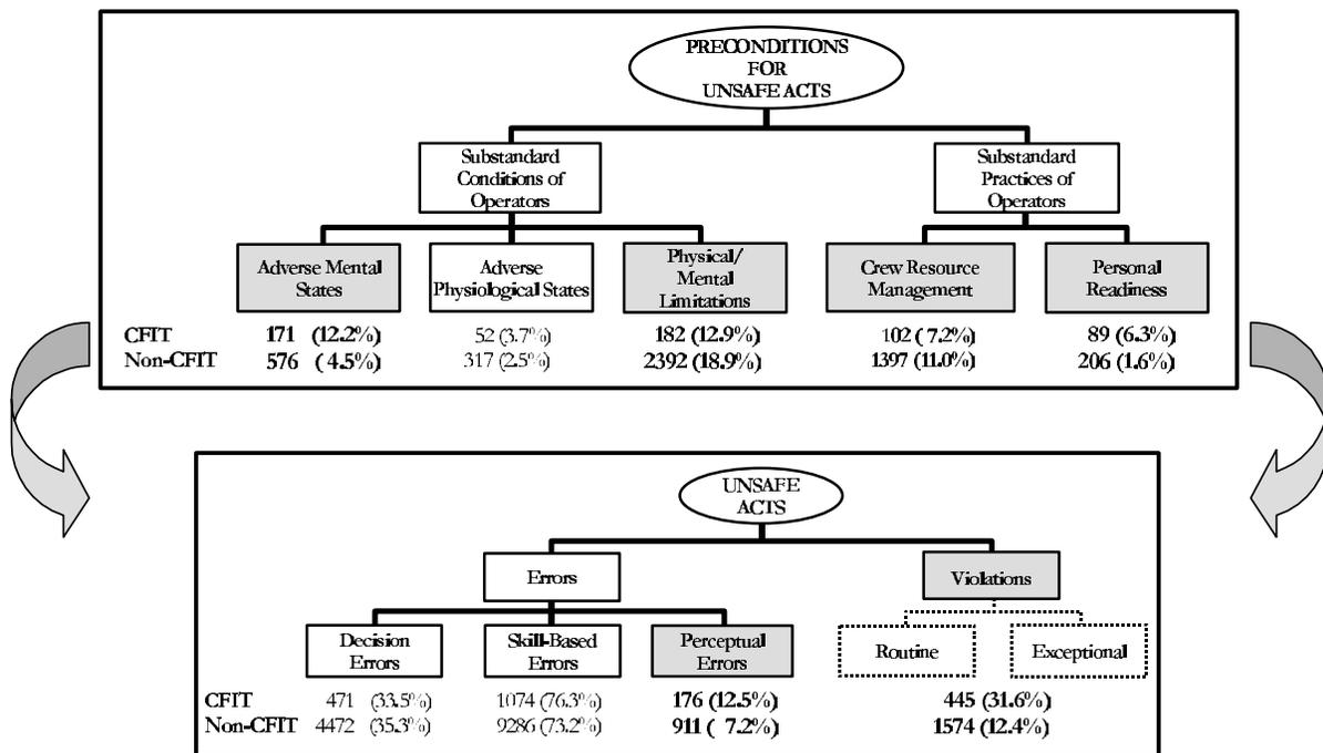
**Figure 3.** Number and percentage of CFIT and non-CFIT accidents associated with at least one instance of each particular causal category. Statistics associated with violations have been collapsed across the type of violation committed. Significant differences ( $p < .001$ ) are represented by shaded boxes.
