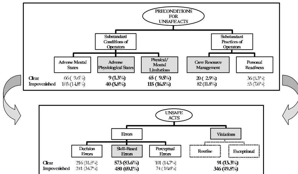
**Figure 5.** Percentage of CFIT accidents occurring in clear versus visually impoverished conditions associated with at least one instance of each particular causal category. Statistics associated with violations have been collapsed across type of violation committed. Significant differences ( $p < .001$ ) are represented by shaded boxes.
