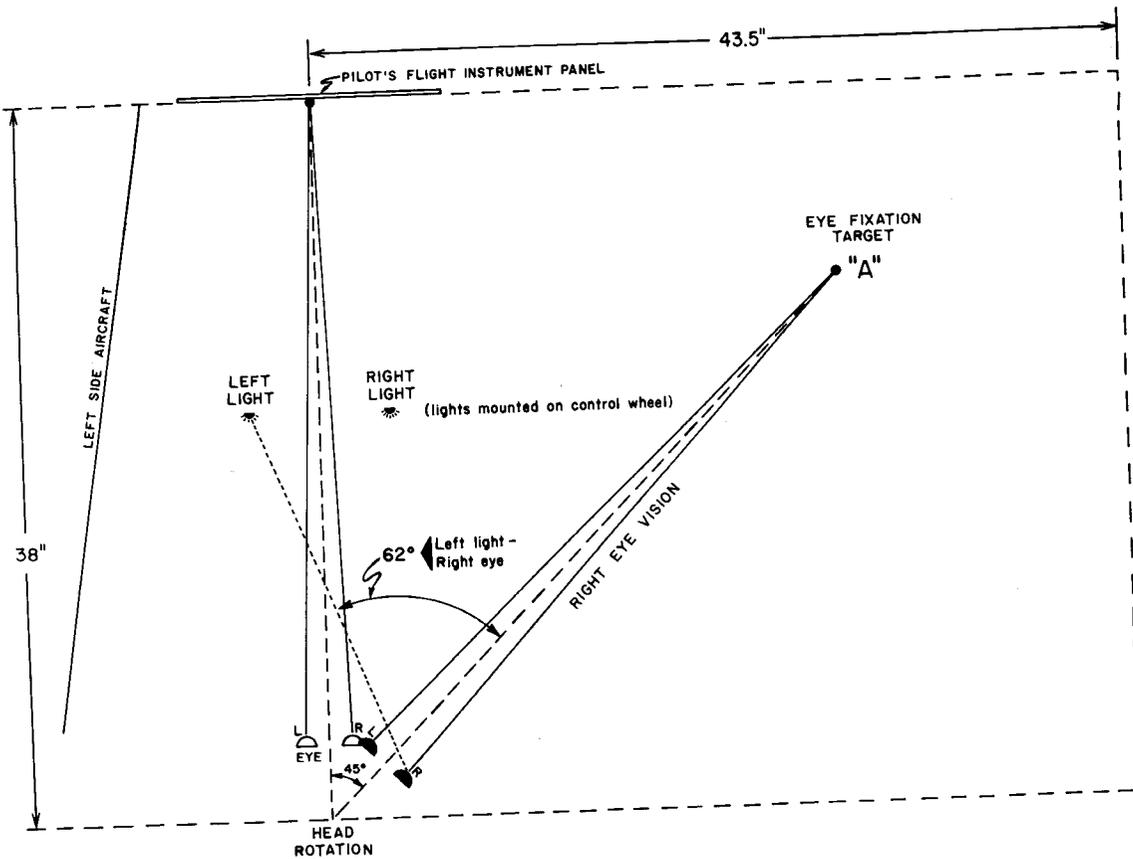
FIGURE 18. Head rotation and angle of peripheral cue discrimination (right eye); lateral discrimination of peripheral cues (Figure 17) was a maximum of 62° for the right eye when fixated to the right.
